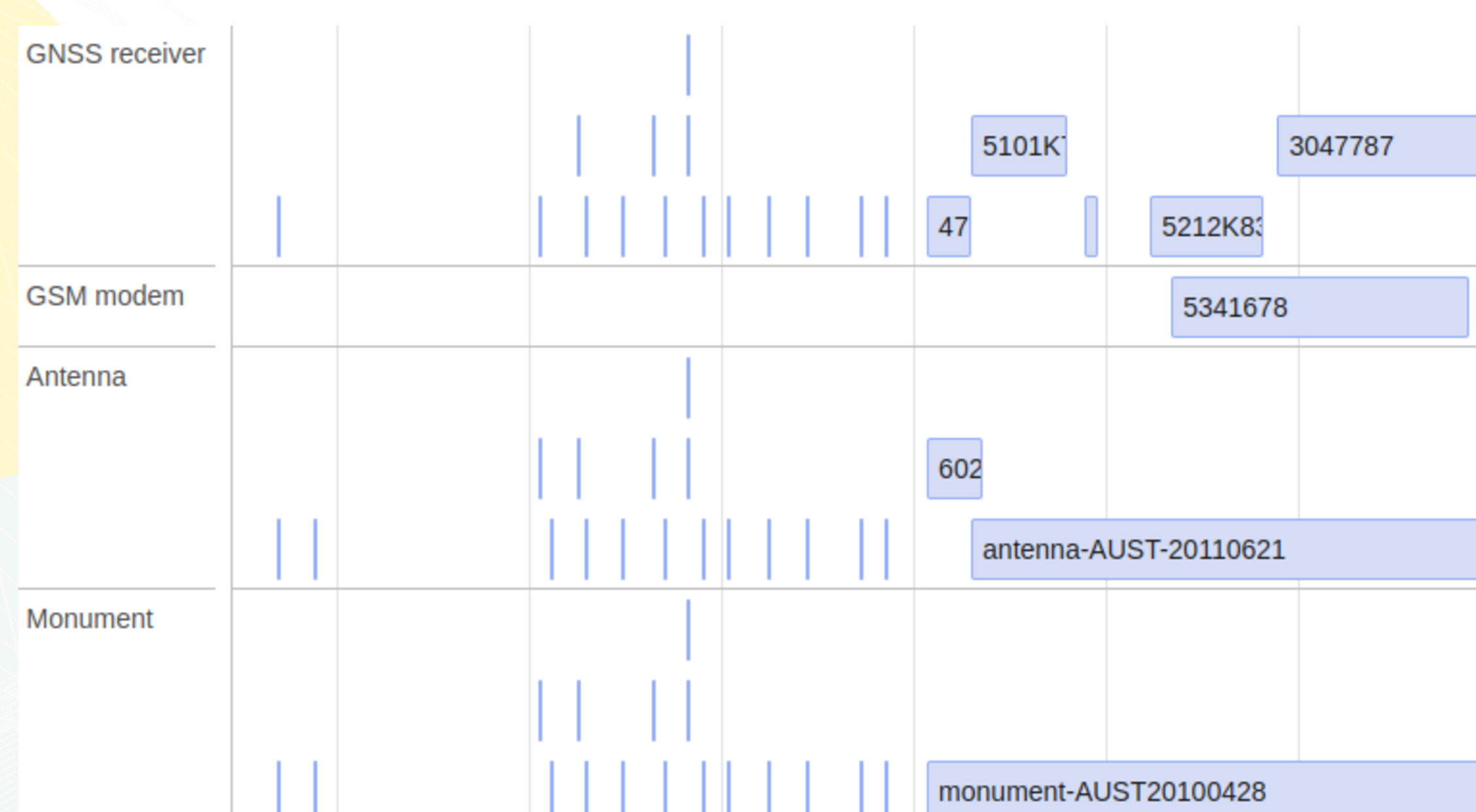
Device history of cGNSS station AUST, located on top of Katla volcano. The timeline shows frequent equipment changes over the years, including multiple GNSS receivers, and antennas. Stations with long and complicated histories like this require detailed metadata review and reconstruction before they can meet EPOS metadata standards.
