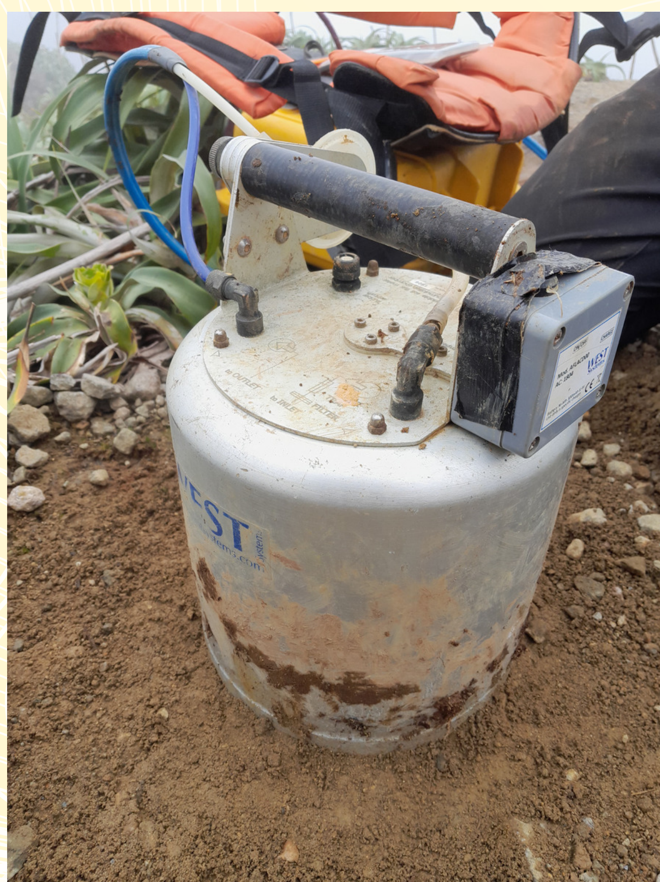
Accumulation chamber for CO 2 flux measurements
